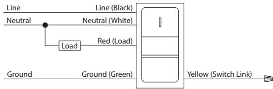
VS 1 (Master / Master) Three-way Wiring - up to maximum 4 sensors can be grouped via "Switch Link"
